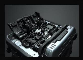
The fiber retention clamps support the automated operations. When the sheath clamps open automatically after splicing, the fiber retention clamps gently hold the spliced fiber to keep it from flying out. The retention clamps release when the fiber is lifted by the operator.
